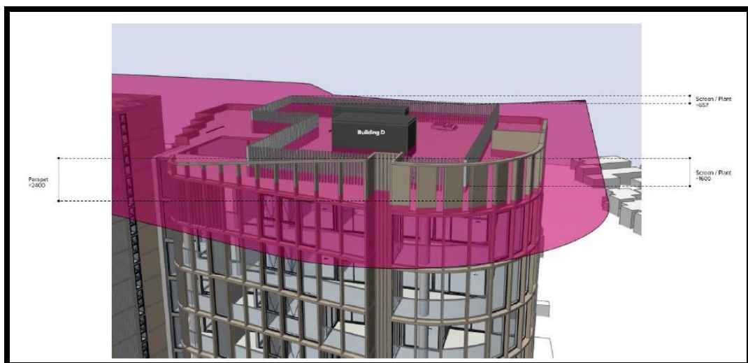
Figure 14: Height plan drawing which illustrates the components which are above the height control for Building D (Source: Turner).
